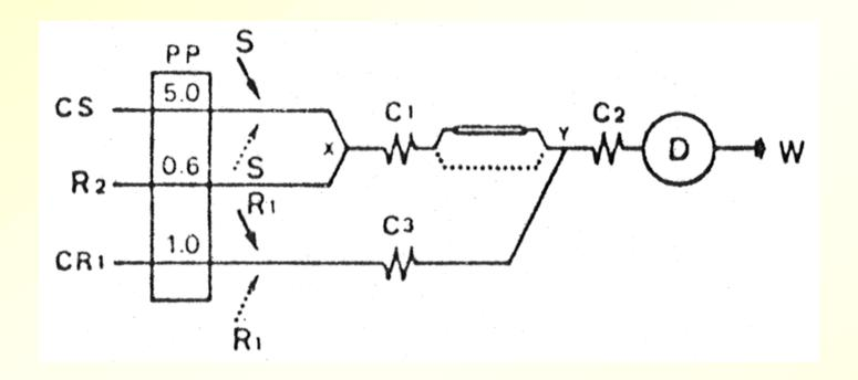
$C_s$ (water) and  $C_{R1}$  (phosphoric acid) = carrier streams for the sample (S) and color-forming reagent ( $R_1$ )
