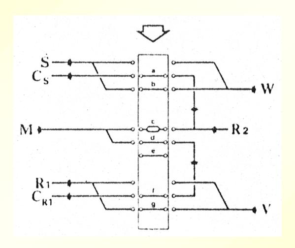
a, b = sampling loops; c = reducing column; d, e = connectors; f, g = reagent loops; M = manifold
