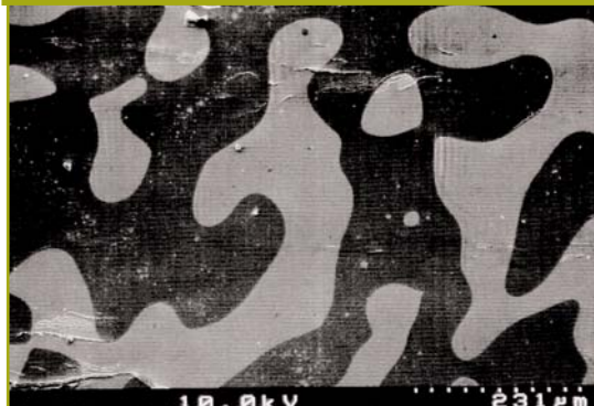
Scanning electron micrograph of the annealed P \alpha MSAN/PMMA 40/60 blend. Crack propagation velocity: 10–5 mm/cycle. (Magnification: 130x)
