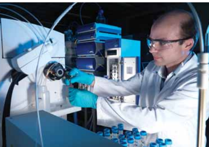
FFF-ICP-MS is used to determine the size distribution and elemental composition of nanoparticles in food and consumer products. Image courtesy of Andrew Brookes < www.andrewbrookes.co.uk >.
