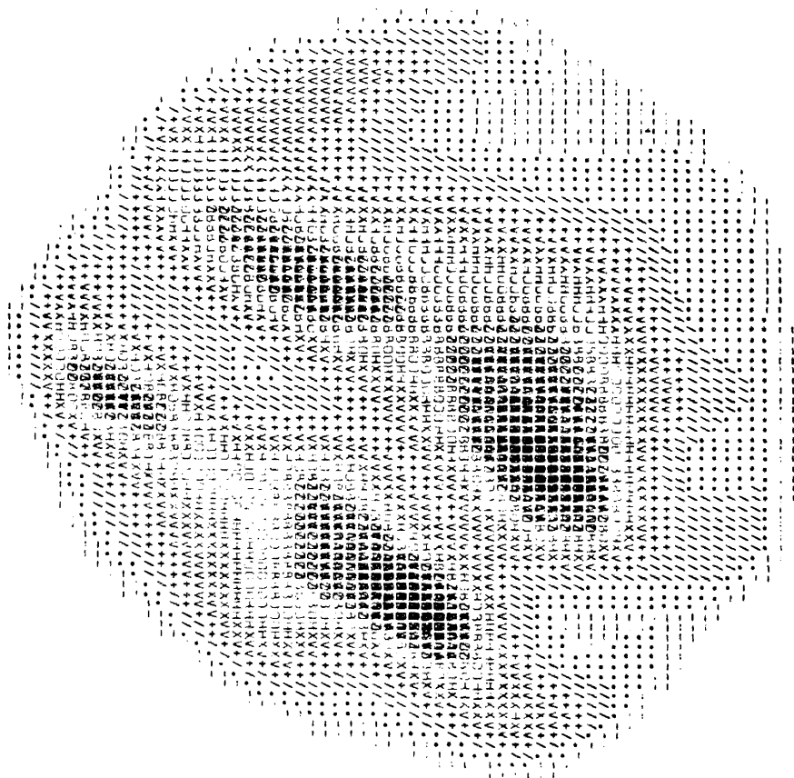
Figure 3. Proton n.m.r. zeugmatogram of the oil distribution within an intact pecan nut ( Carya illinoensis ).
