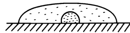
Fig. 7. Types of meniscus boundaries: (a) Soap film, (b) Thin liquid film, (c) Fixed boundary; radius controlled, (d) Moving boundary contact angle controlled.
