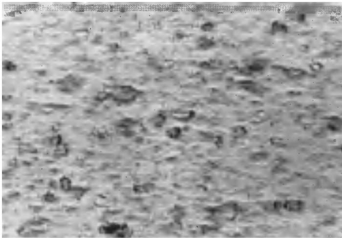
Fig. 4. Filled PVC with 10 % coarse \text{CaCO}_3
