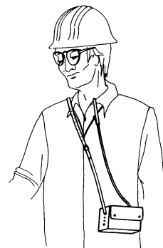
Fig. 13. Long-term measurements at work-places by means of detector tubes (personal monitoring)
