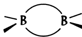
Fig. 2. Structure of B 2 H 6 . A bridge hydrogen is represented by a curved line, and a terminal hydrogen is indicated by a straight line.
