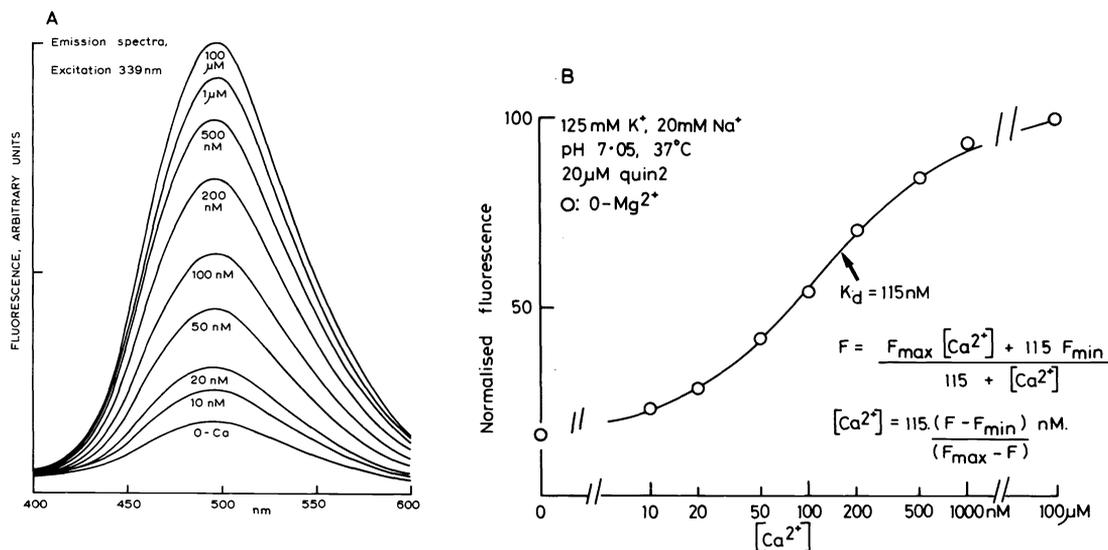
Fig. 4. Fluorescence response of quin2 to  $[Ca^{2+}]_i$ . A, shows emission spectra from 20  $\mu M$  quin2, in a background at 125 mM  $K^+$  and 1 mM free ( $Mg^{2+}$ ) and pH 7.05. The procedure for altering ( $Ca^{2+}$ ) is given in Ref. 27. B plots the signal at 492 nm against  $[Ca^{2+}]$ . The data fit well to a simple 1:1 binding relation shown in the Figure. The solid line is the theoretical curve for an apparent  $K_d = 115$  nM.
