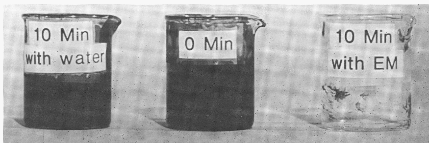
Fig. 3. Removal of adhering oil from solid surfaces with EM.
