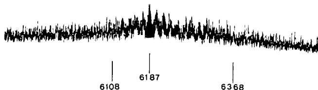
Fig. 4: Molecular ion region of a permethylated GSL with 25 sugar residues obtained from a thioglycerol matrix by FAB MS using a V.G. ZAB HF instrument. Mass determination of the center of the most intense ion cluster was performed by interpolation of C_{s_n}J_{x-1}^+ ions.
