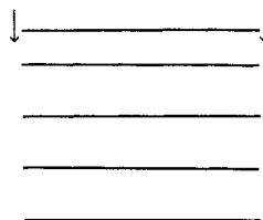
Fig. 2. Shortened interlayer spacing between the first and second layer of atoms at the surface.
