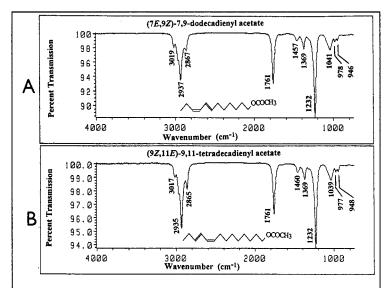
Fig. 4.. Gas phase infrared spectra of (7E,9Z)-7,9-dodecadienyl acetate (**A**), and (9Z,11E)-9,11-tetradecadienyl acetate (**B**) (resolution=8 cm<sup>-1</sup>).
