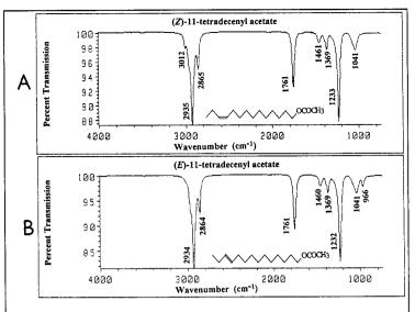
Fig. 1 Gas phase infrared spectra of (Z)-11-tetradecenyl acetate (A), and (E)-11-tetradecenyl acetate (B) (resolution= 8 cm<sup>-1</sup>).
