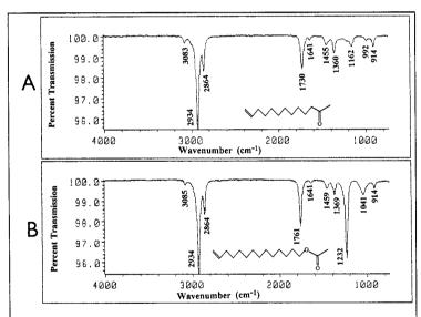
Fig. 2. Gas phase infrared spectra of 12-tridecen-2-one (A) and 13-tetradecenyl acetate (B) (resolution=  $8 \text{ cm}^{-1}$ ).
