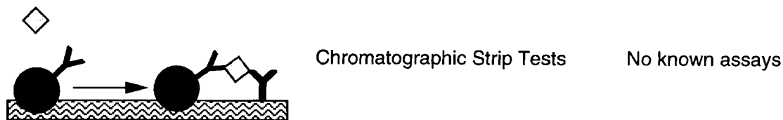
Fig. 4 "One Step" strip or chromatographic tests and assays. First antibody-coated, dyed microspheres migrate along strip to immobilized second antibody; antigen sandwich forms colored line.
