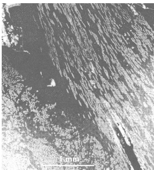
Figure 6. The interface between the die entry cone (streamline flow) on the right hand side and recirculation zone (left) shown at higher magnification using scanning electron microscopy. Some voids are present owing to the solidification taking place in the barrel. The lighter coloured glass fibres are shown against the darker polypropylene background.
