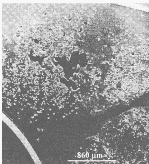
Figure 4. The fibre dispersion through the granule cross section, showing inhomogeneity.
