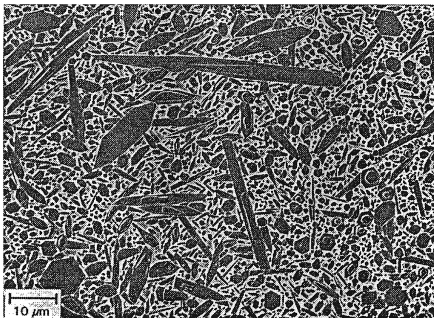
Fig. 1 Scanning electron micrograph of a gas-pressure sintered silicon nitride ceramic after plasma etching. The micrograph shows elongated \text{Si}_3\text{N}_4 grains embedded in a matrix of fine, equiaxed grains and a grain-boundary phase (reproduced from ref. 80).
