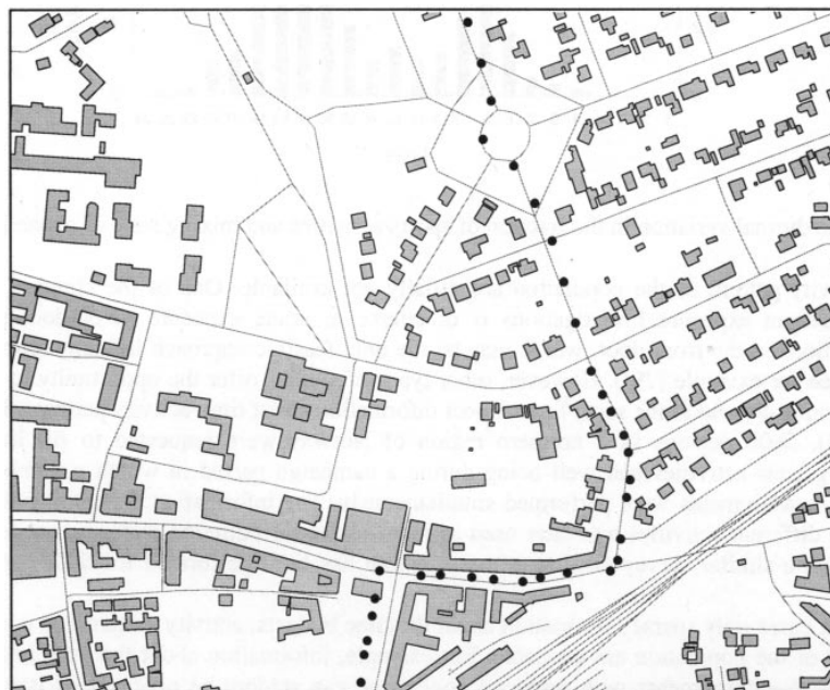
Fig. 10 Example of GPS data logging during an air pollution exposure study in Denmark. Positions are plotted as black dots for every 6 s. Data are obtained from a GPS in a backpack, and an adjustment is performed by use of a corrector that makes use of information from FM radio-masts with known positions (differential GPS).
