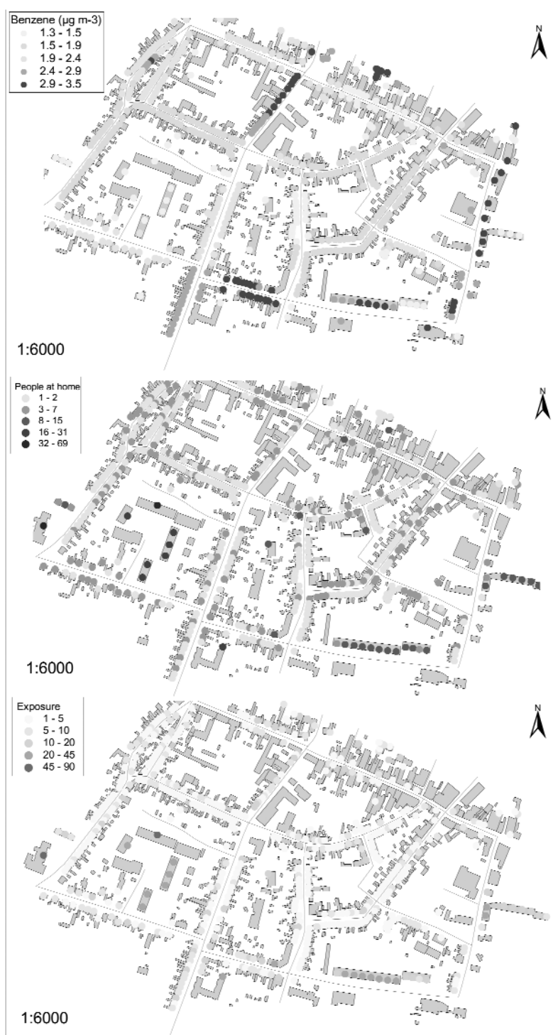
Fig. 8 Number of people living at a given address, annual mean benzene concentrations (1996) computed with the AirGIS model, and a simple exposure index given by number of people multiplied by the annual mean concentration [86].
