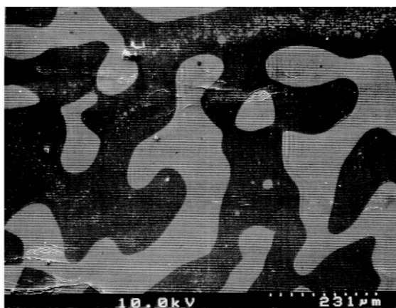
Fig. 25 Scanning electron micrograph of the annealed P \alpha MSAN/PMMA 40/60 blend. Crack propagation velocity: 10 -5 mm/cycle. (Magnification: 130 \times )
