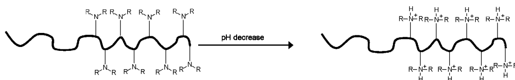
Fig. 2 Change in solubility upon protonation of a copolymer having weakly basic amines in one block.
